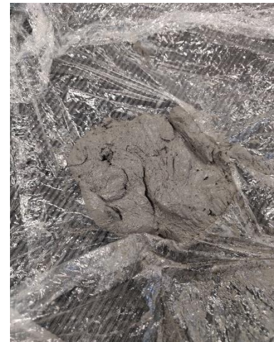
Figure 4. A completely remoulded sample after hand kneading
