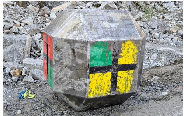
Figure 5. Steel armoured test block
