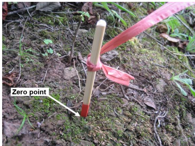
Figure 4. Bamboo stake installed to measure shoreline erosion on Three Gorges Reservoir. Photo from Xiaolei Su.
