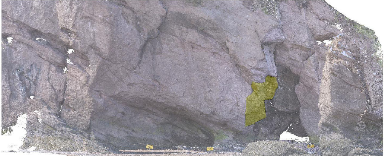
Figure 2. Preliminary 3D photogrammetry model of the cliff with the failure surface highlighted in yellow. Note that this model is a separate, lower resolution model compared to the models in Figures 3 & 4, and the yellow signs in the foreground are 75 cm x 30 cm each for scale.
