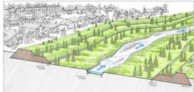
Figure 55 Schematic example of debris flood mitigation using a wide flood plain with setback berms (artwork by D. Shuttleworth, image provided by BGC Engineering Inc.).
